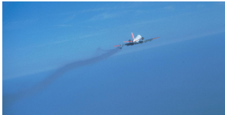
Fig. 17 ATTAS seen from behind. Effect of oscillating flaps on smoke trace
