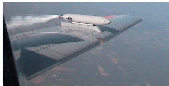
Fig. 16b The smoke generator on the ATTAS wing
