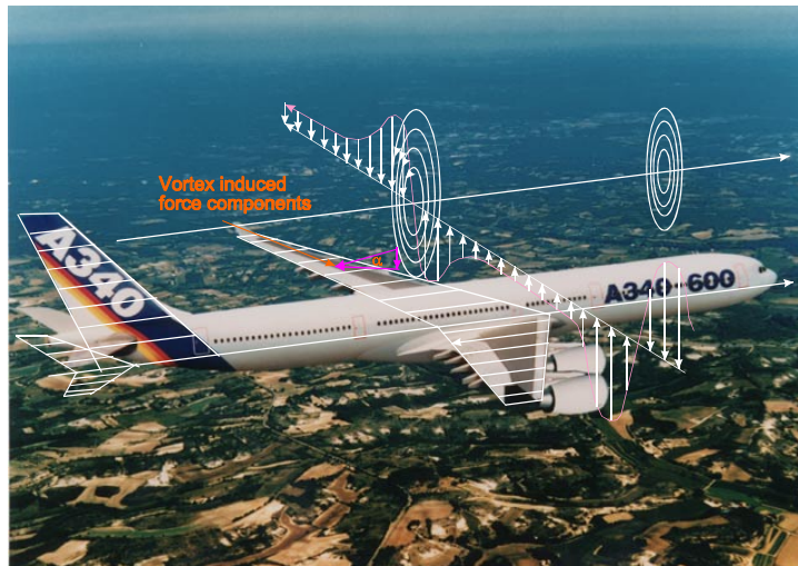
Fig. 14 Strip Method: Horizontal and vertical surfaces of the aircraft are divided into a number of lift generating strips
