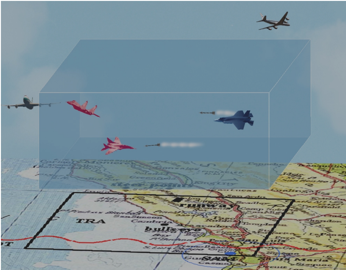
Figure A.1: Airspace temporarily reserved for Embedded Training – Virtual adversaries and missiles are generated in simulation equipment on-board the own ship (on the right-hand side in the reserved airspace).
