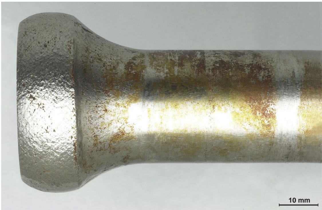
Fig. 4 Two similar views of the rod ends that were seated in the connectors
