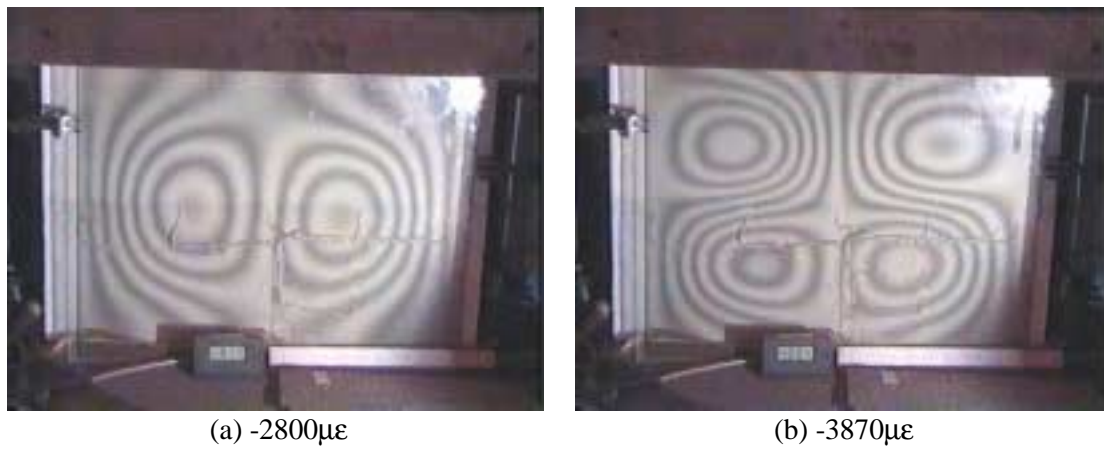
Figure 7 – Front face Moiré of DR2 after bay impact
