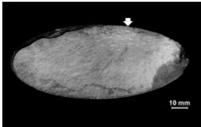
Fig. 2 Macro photograph of the yellow arm outboard fracture surface. The failure origin is arrowed
