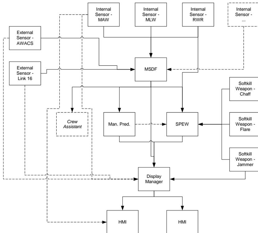
Figure 2: Multi-Agent System overview; dotted lines represent alternative information flow when components fail
