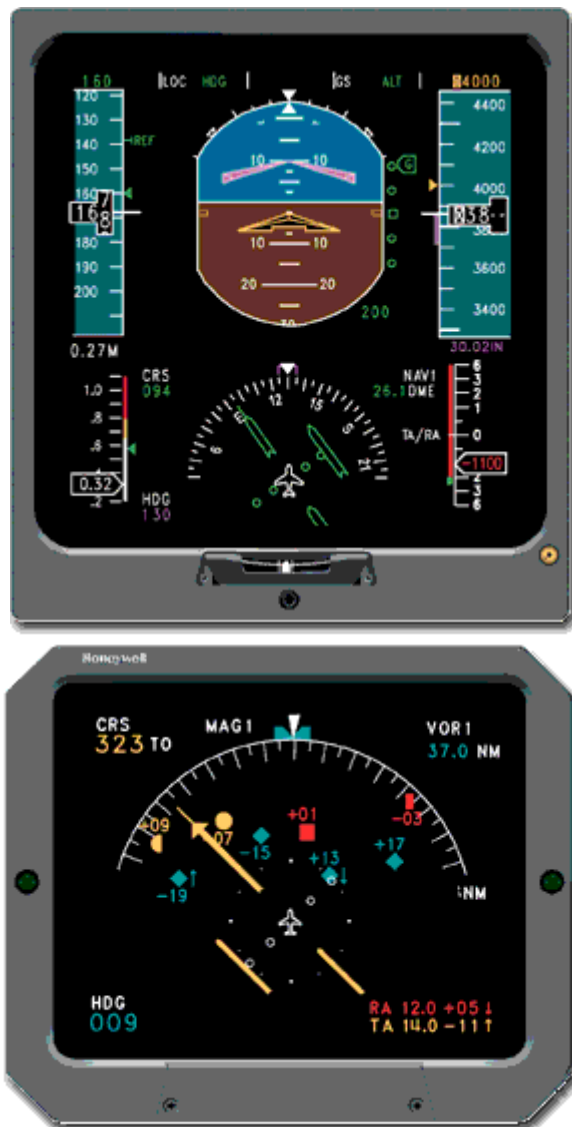
figure 6.2 Example of a TCAS displays (Honeywell TCAS 2000 display)
