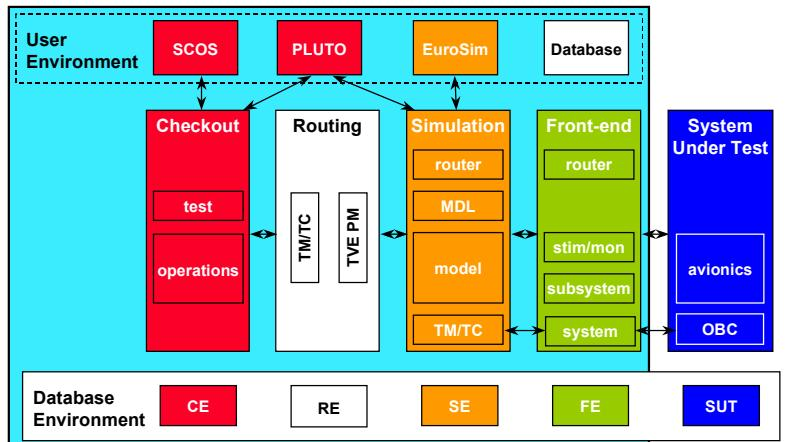
Fig. 6. Conceptual architecture of the next generation Test and Verification Equipment, showing the main elements and interfaces
