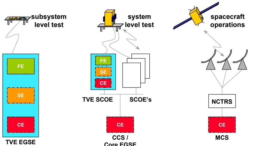
Fig. 5. System commonality for avionics subsystem level tests, avionics tests at system level and spacecraft operations
