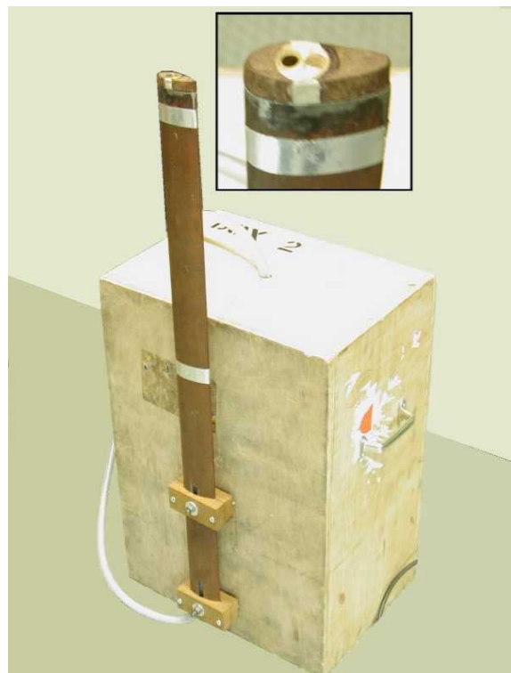
Fig. 2 Reference source with monopole sound radiation
