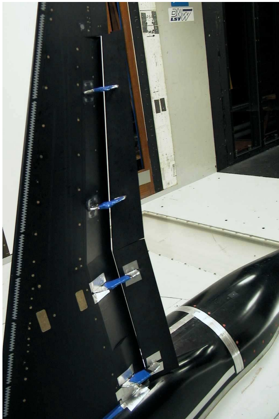
Fig. 3 Aircraft model view from wing pressure side (“clean” landing configuration)
