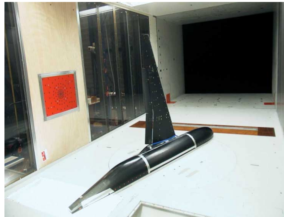
Fig. 1 Aircraft model and acoustic array in the DNV-LST test section
