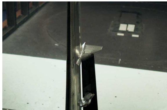
Fig. 4 Details of the flap tip fence (upper plus lower fence) on the aircraft model (flaps removed on upper photo)
