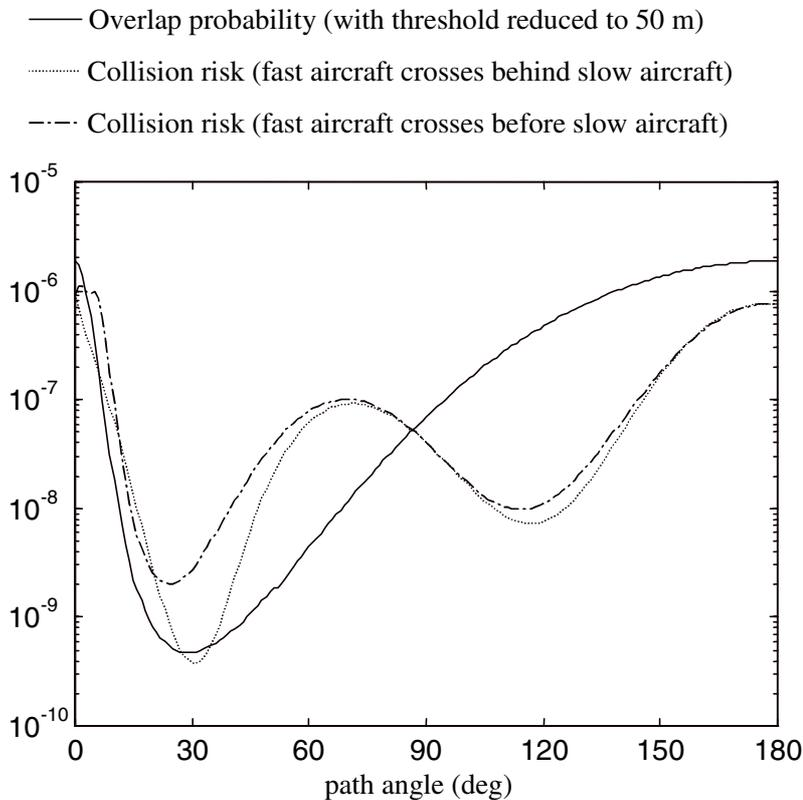
**Figure 11: Difference between situations in which a faster aircraft crosses before or after a slower aircraft. Evaluated overlap probability (with threshold reduced to 50 m) and collision risk are shown.**
