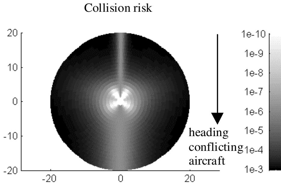
**Figure 9: Collision risk is represented by colours for various path angles and times to minimum predicted separation.**
