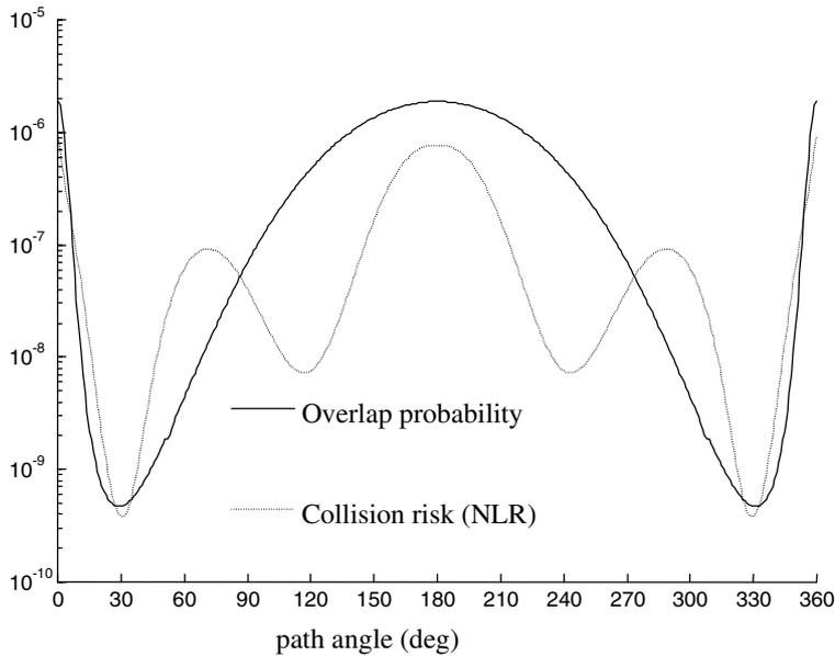
**Figure 10: Overlap probability (with threshold reduced to 50 m) and collision risk for various path angles and 4 minutes before time of minimum predicted separation of 6 n miles.**
