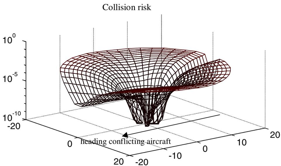
Figure 8: Collision risk (z-axis) is represented for various path angles and times to minimum predicted separation (horizontal axis).
