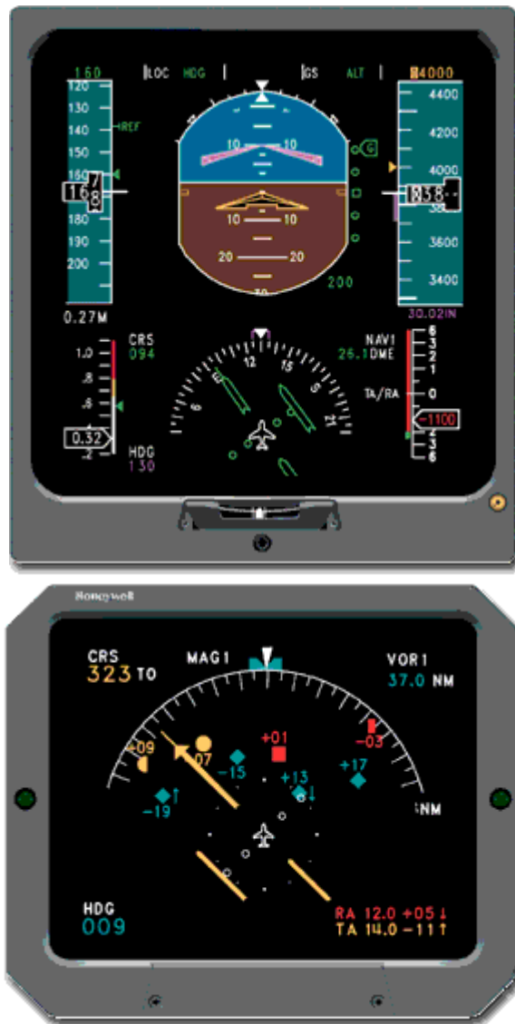
figure 7.2 Example of a TCAS displays (Honeywell TCAS 2000 display)
