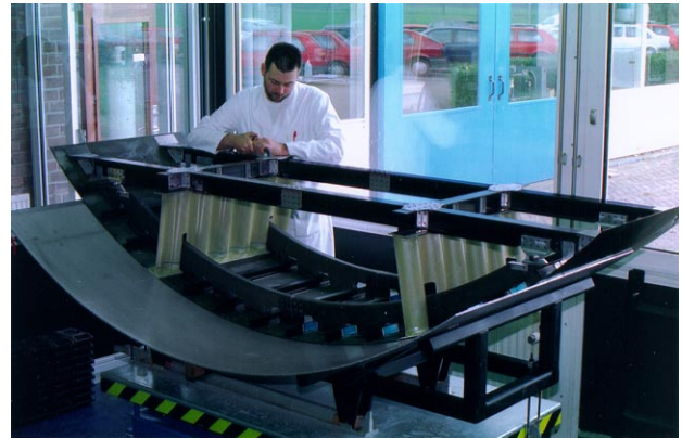
Fig. 8 Final assembly of commuter sub-floor structure (NLR)
