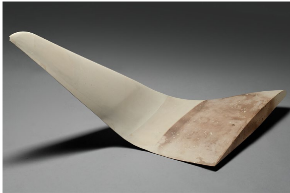
Figure 13: Aramid foam core after machining and sanding
