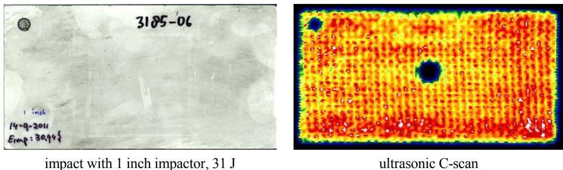
**Fig. 9 Non-detectable high-velocity impact damage on a 20 mm thick, painted RTM specimen [6]**
