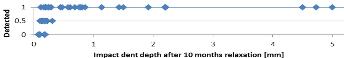
**Fig. 5 Visual inspection of 43 low-velocity impacts on the composite specimens of the NTP project [4] (1: 28 impacts detected, 0.5: 10 impact areas marked as suspect, 0: 5 impacts not detected)**
