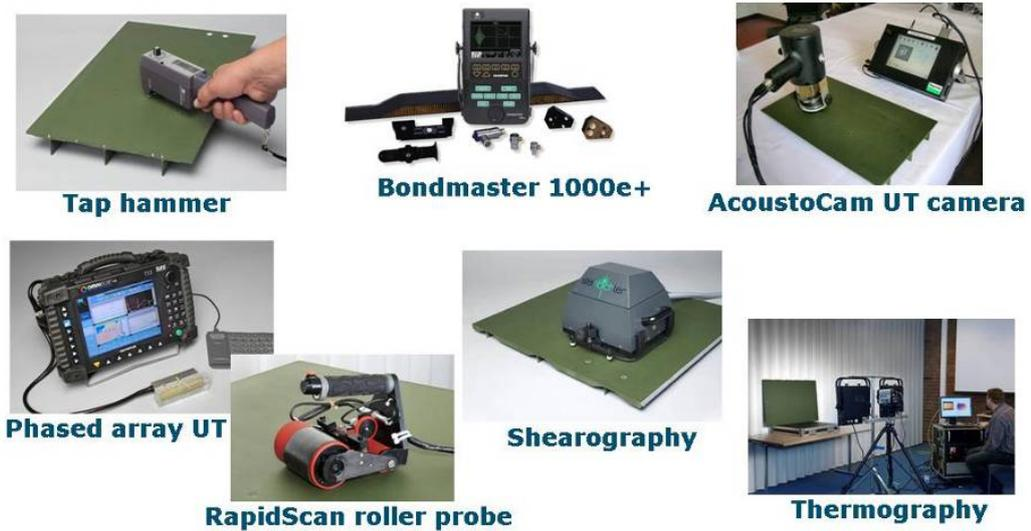
Fig. 4 Selected in-service NDI methods for inclusion in the NTP inspection programme
