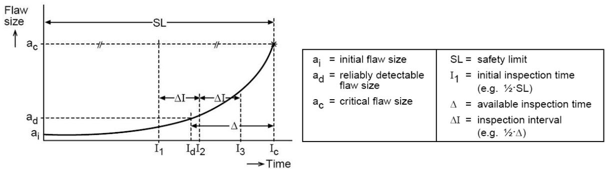
**Fig. 1 Damage tolerance approach for inspectable structures (Fig. 1 from [2])**
