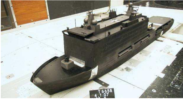
Figure 8. Wind tunnel model of the LPD-2 ‘Johan de Witt’ in the DNW-LST wind tunnel.
