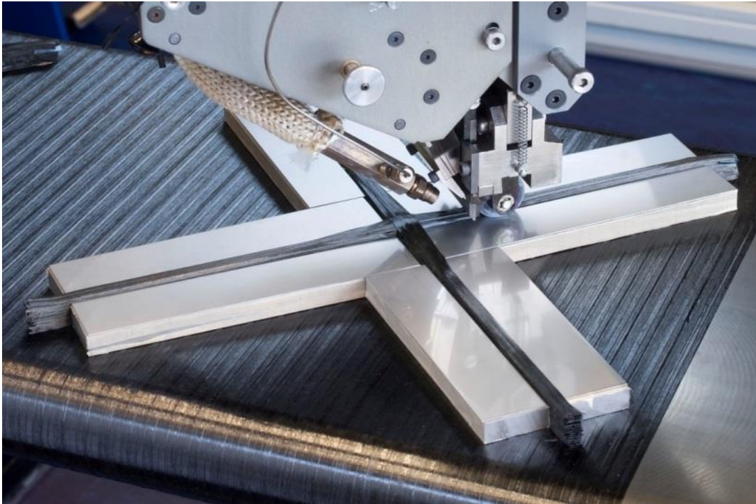
Figure 4: Grid intersection manufacturing with metal support blocks
