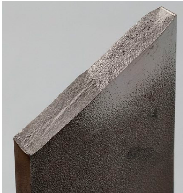
Figure 3. Fracture surface of CA loaded SET specimen, from right to left showing the notch, the pre-crack, the slanted fatigue crack and the final rupture surface.
