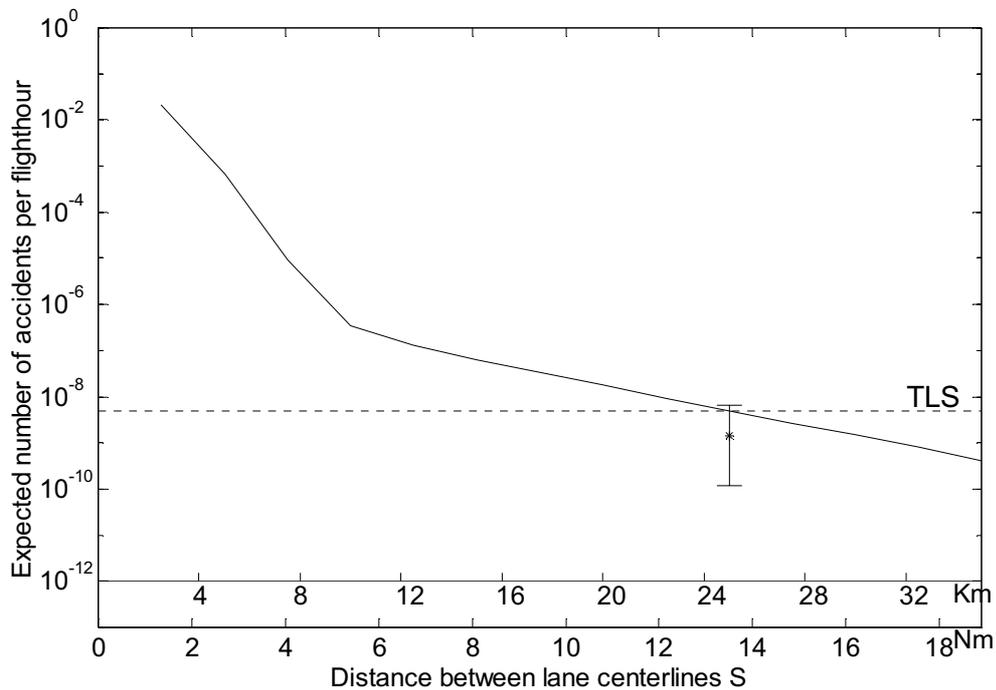
Figure 7 ATC routine monitoring model-based accident risk curve (continuous line) and expected accident risk at  $S=13.5$  NM (denoted by \*). The bar indicates the 95% credibility interval at  $S=13.5$  NM. TCAS effect is not taken into account by ICAO TLS and neither included in the curve or the 95% accident risk area.
