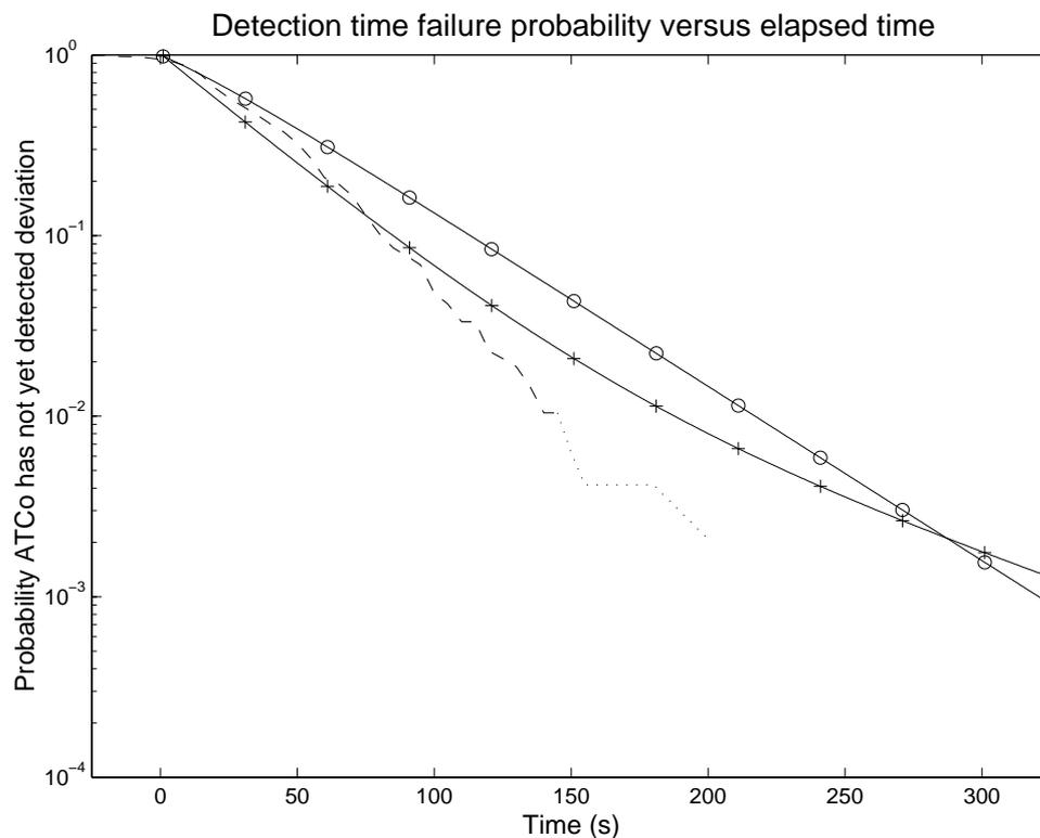
Figure 5 Controller detection time of severe deviations of the full model (line marked '+'), of the reduced model (line marked 'o') and of statistical data (George et al., 1973) (dashed/dotted line, the dotted part representing data based on less than 5 measurements).
