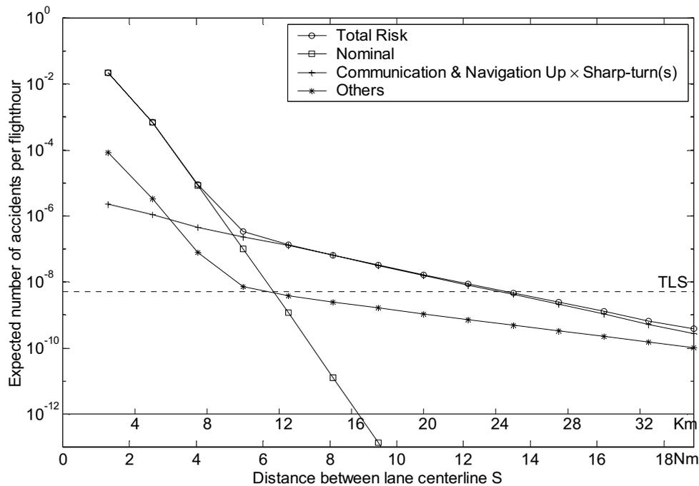
Figure 6 ATC routine monitoring model-based accident risk curve. The horizontal line is the Target Level of Safety (TLS) of (ICAO, 1998). See the main text for an explanation of the curves.
