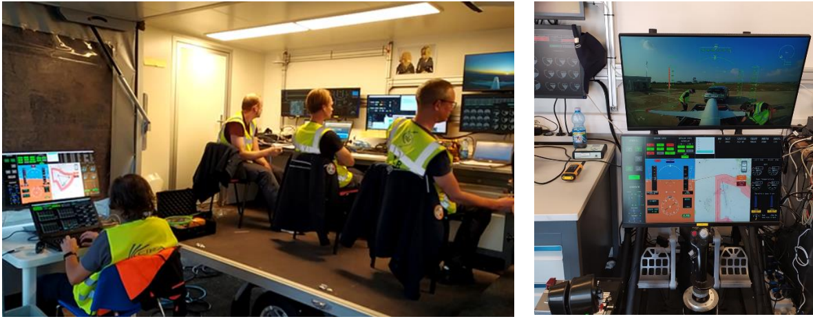
Figure 6 : View of the Ground Remote Pilot Station including the pilot cockpit (right) during operations
