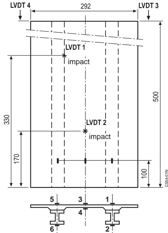
Fig. 5 Compression test panel with locations of impact, strain gauges and LVDT's
