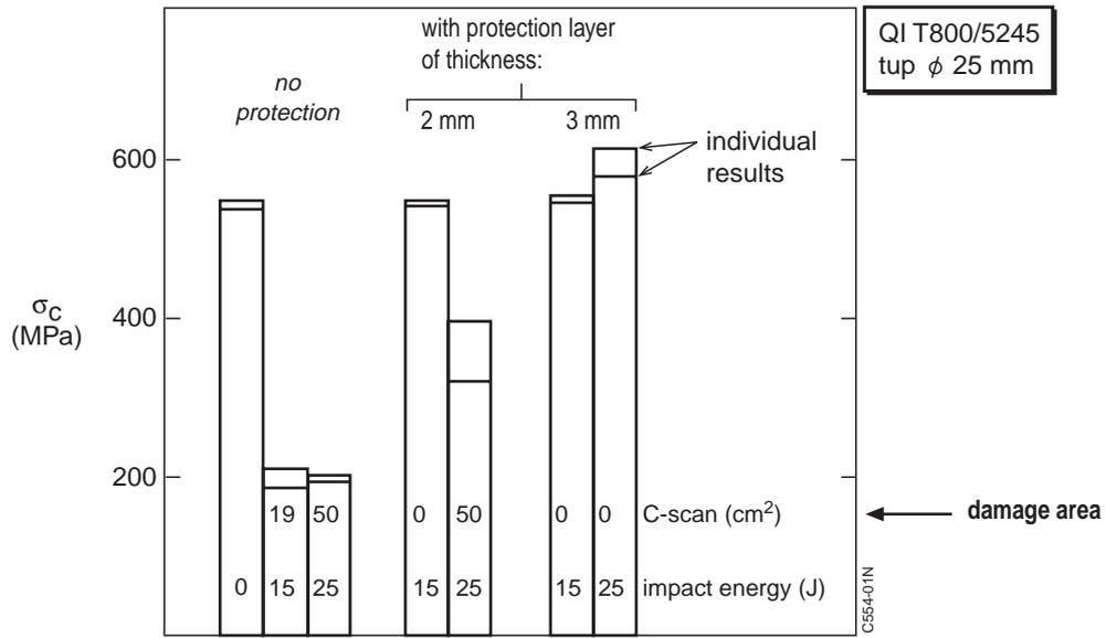
Fig. 3 Compression after impact strength of a 4 mm thick quasi-isotropic 110 mm wide coupon specimen tested in an anti-buckling guide
