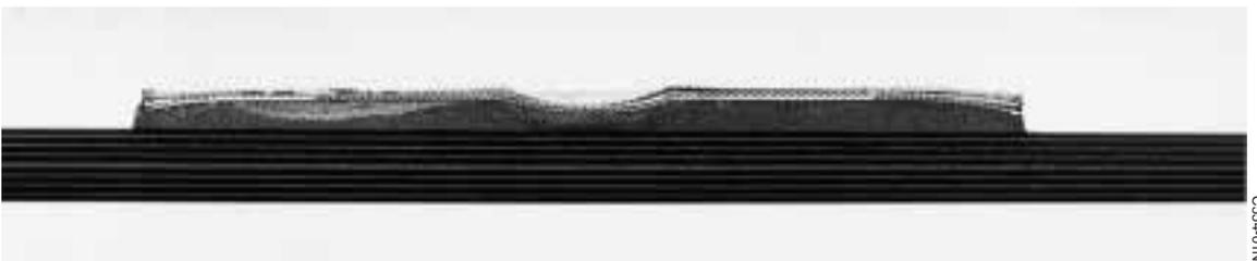
Fig. 2 Cross sections of impacted 4 mm thick carbon/epoxy specimens
