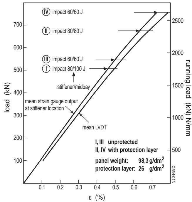
Fig. 6 Load - strain behaviour of tested compression panels and failure loads
