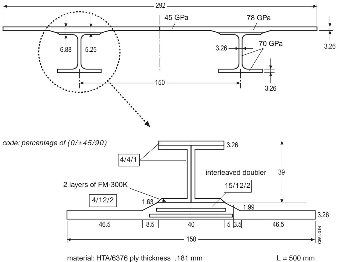
Fig. 4 Dimensions of compression test panel and lay-up details
