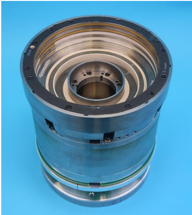
Figure 8. RDAS rotor showing contactless transfer. At the bottom: pedestal and hub simulator.
