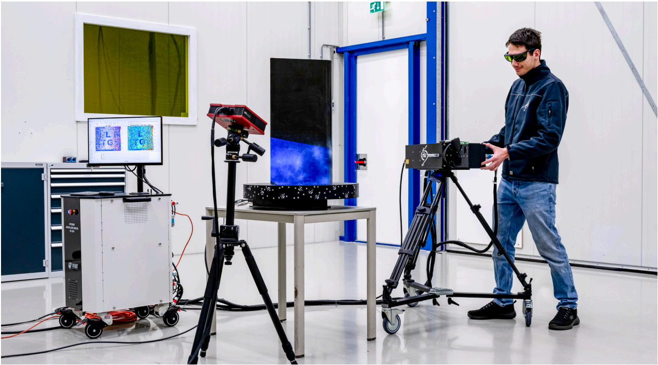
Figure 7. The NLR integrated LUT system with the following components from left to right: PC with software, the Zeiss Atos 5 3D scanner, a curved component standing on the marked rotation table and the laser ultrasonic scanner [15].
