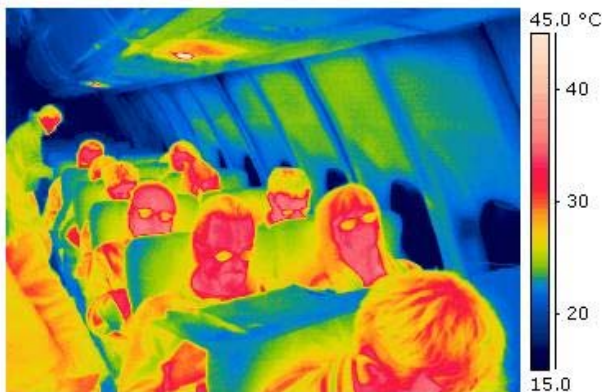
Infrared measurement of passenger surface temperature in an aircraft cabin (Copyright Fraunhofer IBP).
