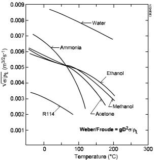
Figure 4.  $(\sigma/\rho_l)^{\frac{1}{2}} = D.g^{\frac{1}{2}}.(We/Fr)^{\frac{1}{2}}$  versus temperature, for various fluids
