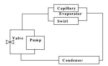
Figure 1. Two-phase loop layout
