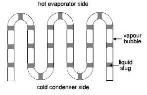
Figure 14. Schematic of an oscillating device section
