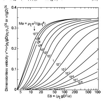
Figure 16. Dimensionless velocity v\* as a function of Morton number Mo and Eötvös number Eö
