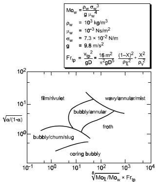
Figure 2. Flow pattern map (vertical downward flow)
