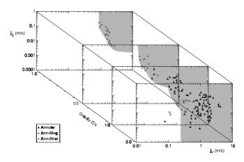
Figure 7. Annular flow: Gravity dependent 3-D map
