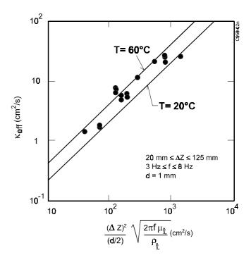
Figure 12. Effective thermal diffusivity
