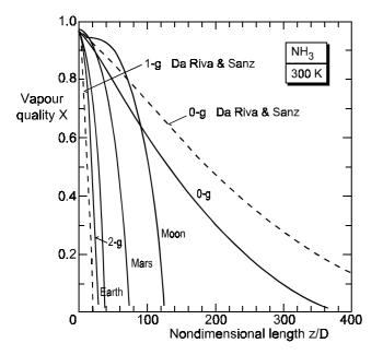
Figure 6. Vapour quality along the reference duct
