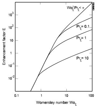
Figure 13. Enhancement factor E as a function of Womersley number Wo<sub>1</sub> and Prandtl number Pr<sub>1</sub>
