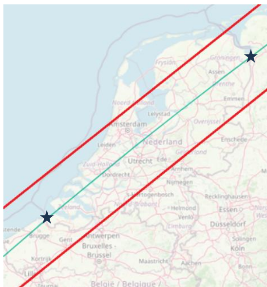
Figure 4: Predicted ground-track of BRIK-II satellite during possible re-entry event. The entry (bottom left) and exit (top right) points over the Netherlands as well as the \pm 35 km buffer are shown with the stars.
