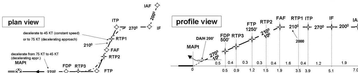
Figure 4 Sketch of generic segmented procedure
