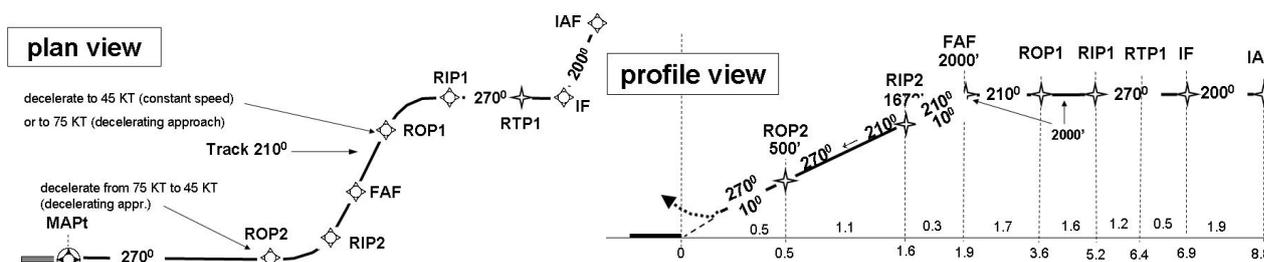
Figure 5 Sketch of steep curved final approach procedure
