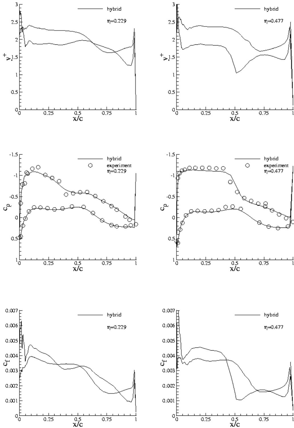
Fig. 11 Comparison of the viscous flow solution and the experiment for the AS28G wing-body; Distribution of  $y^+$ , pressure and skin friction coefficient for the sections 0.229 and 0.477.
