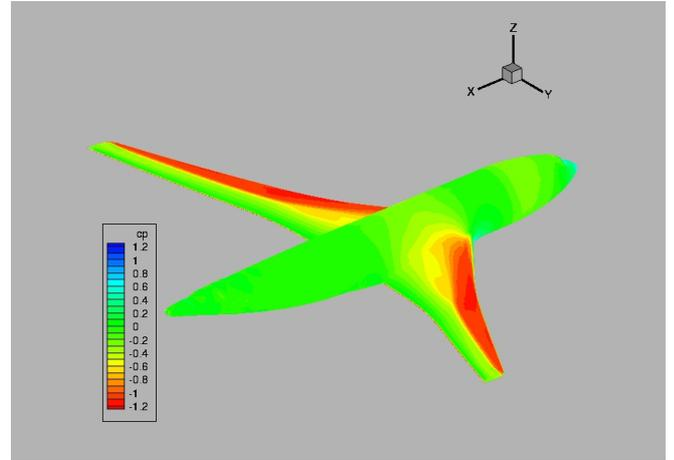
Fig. 9 Pressure distribution for the AS28G wing-body
