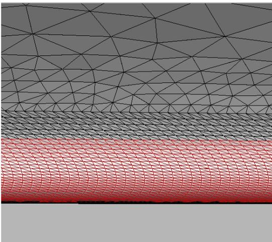
Fig. 8 Specification of the laminar flow region on leading edge of the wing; AS28G wing-body
