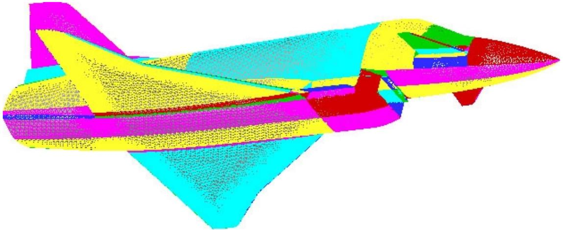
*Fig. 2 Surface triangulation of the CFD-geometry for the X31 experimental aircraft*
