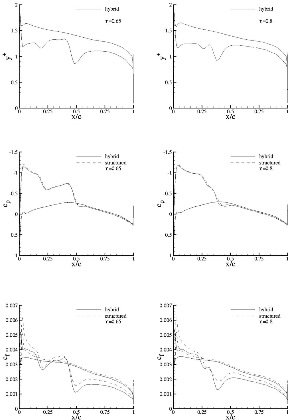
Fig. 7 Comparison of hybrid and structured grid viscous flow solutions for the ONERA M6 wing; Distribution of  $y^+$ , pressure and skin friction coefficient for the sections 0.65 and 0.8.
