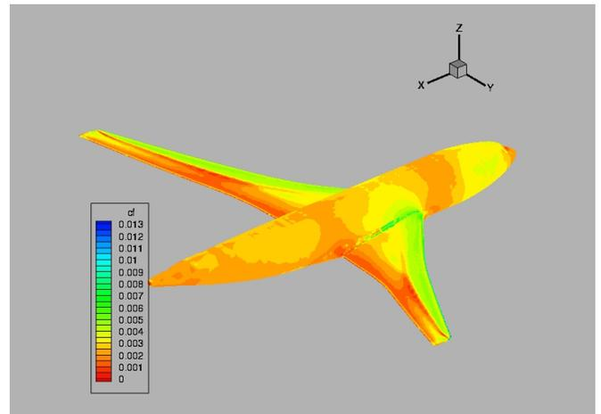
Fig. 10 Skin friction distribution for the AS28G wing body
