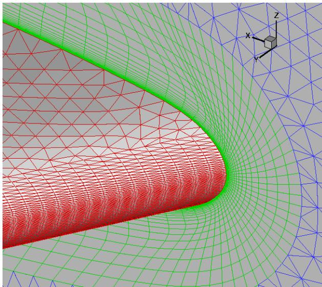
Fig. 4 Surface triangulation of the ONERA M6 wing; close-up of the wing leading edge
