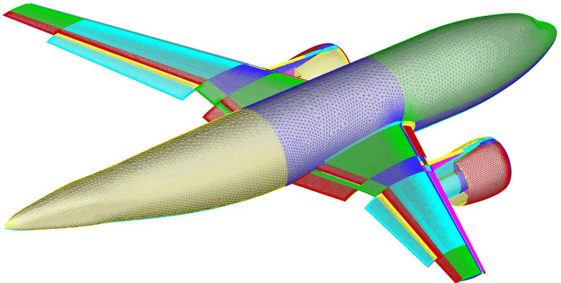
*Fig. 3 Surface triangulation of the CFD geometry for the ALVAST high-lift configuration*
