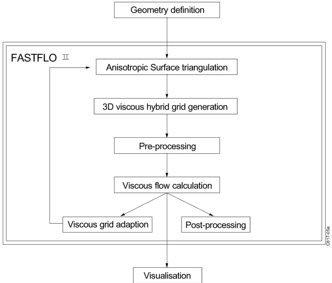
Fig. 1 Overview of the algorithmic components in the FASTFLO CFD system
