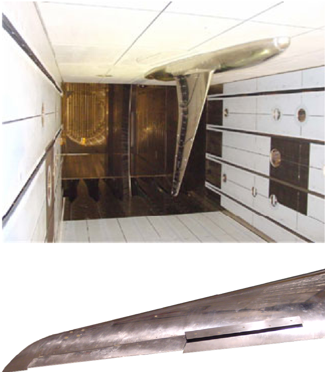
Figure 2: HiReTT N47 semi-span model in the ETW test section (top), and detailed view of outer wing of mla-configuration with upwards deflected mid-board spoiler and aileron (bottom)
