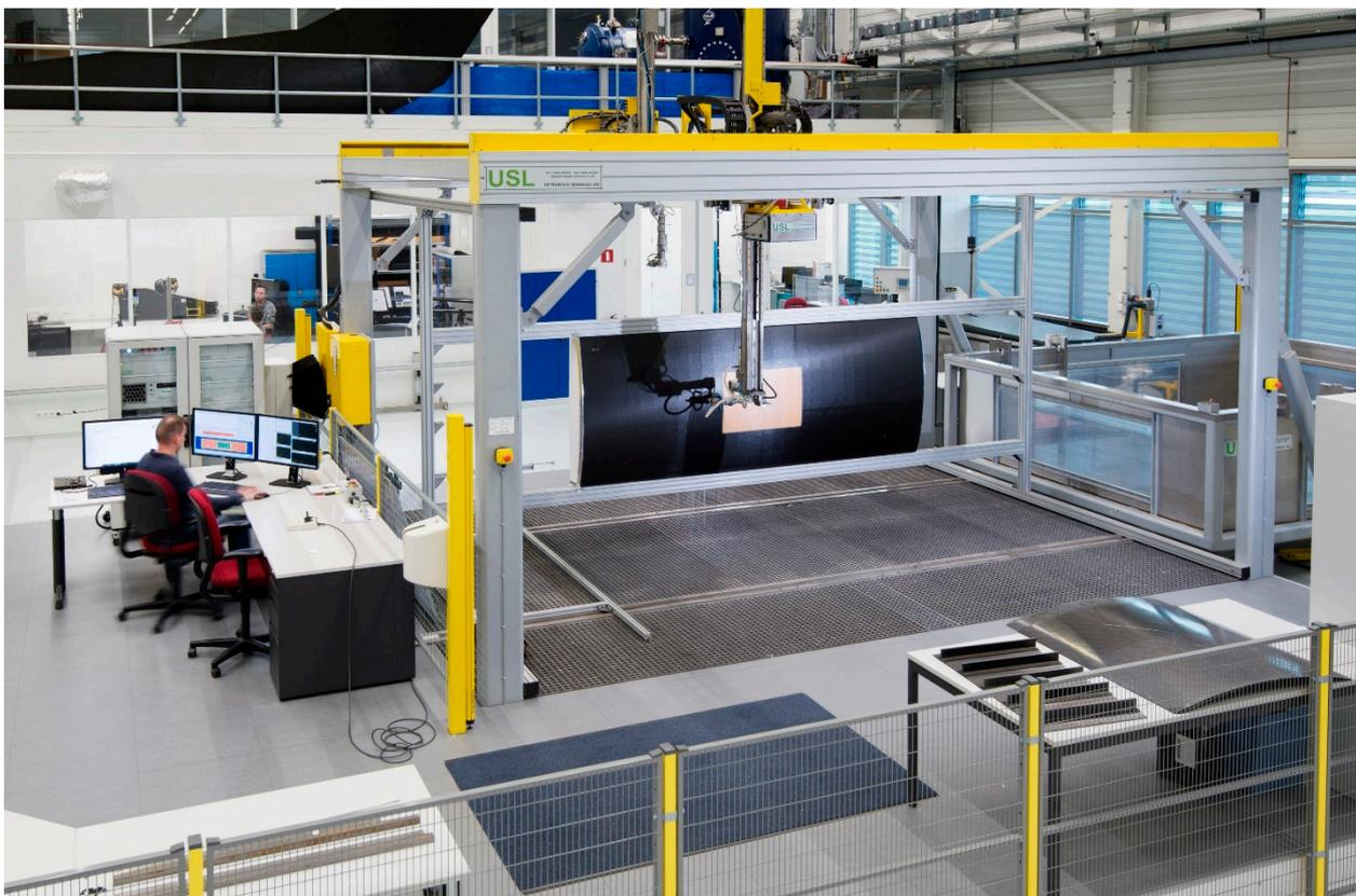
Figure 4.1: Ultrasonic C-scan equipment at NLR
