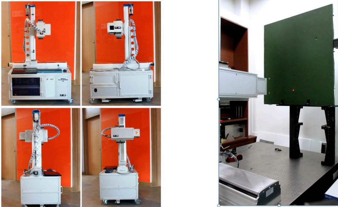
Figure 4.7: PE-UPI system in different views (left) and inspecting specimen NLR-D (right)
