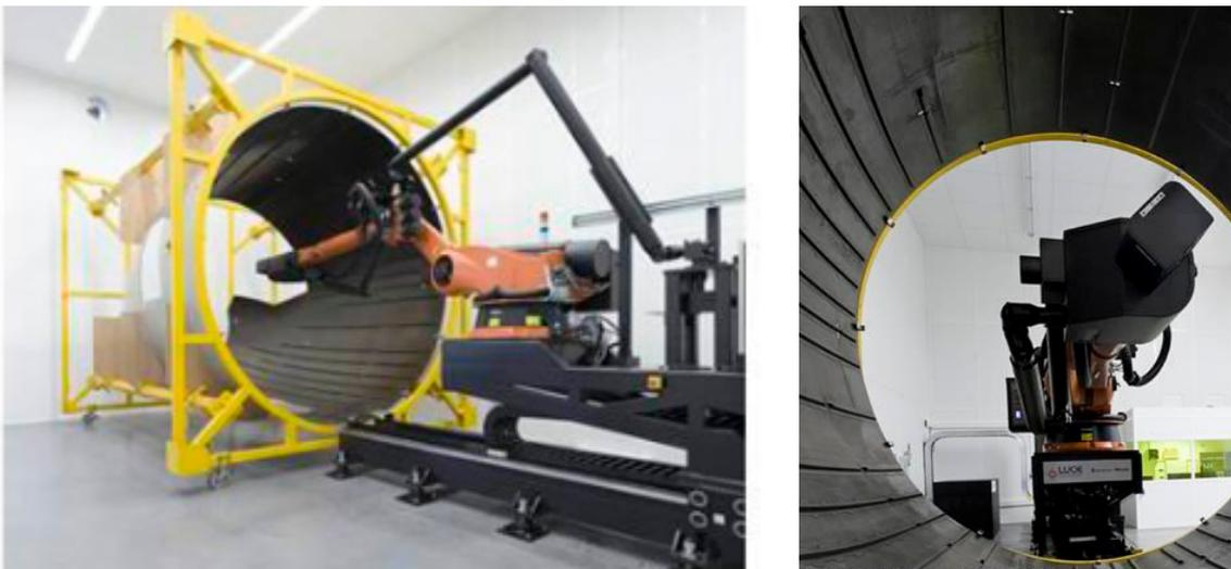
Figure 2.3: LUCIE system of the company Tecnatom S.A. inspecting an Airbus composite fuselage part (Ref. 14)
