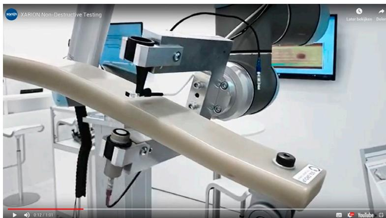
Figure 4.25: The Xarion transmission set-up with aligned excitation laser (under) and optical microphone
