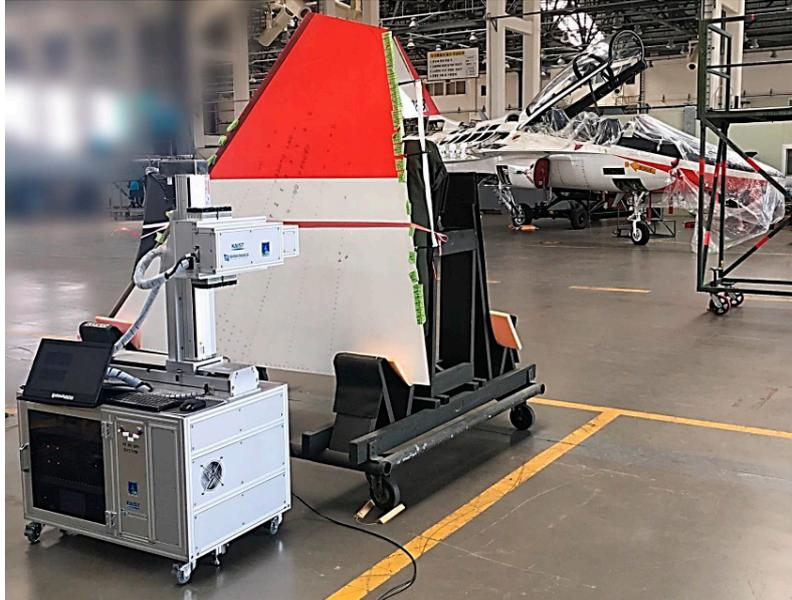
Figure 2.7: PE-UPI laser ultrasonic system of the South Korean company X-NDT. Field inspection of a T-50 horizontal stabilizer (Ref. 21)
