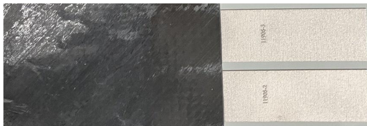
Figure 6: Laminate section with two hot-pressed hybrid titanium-composite joints.
