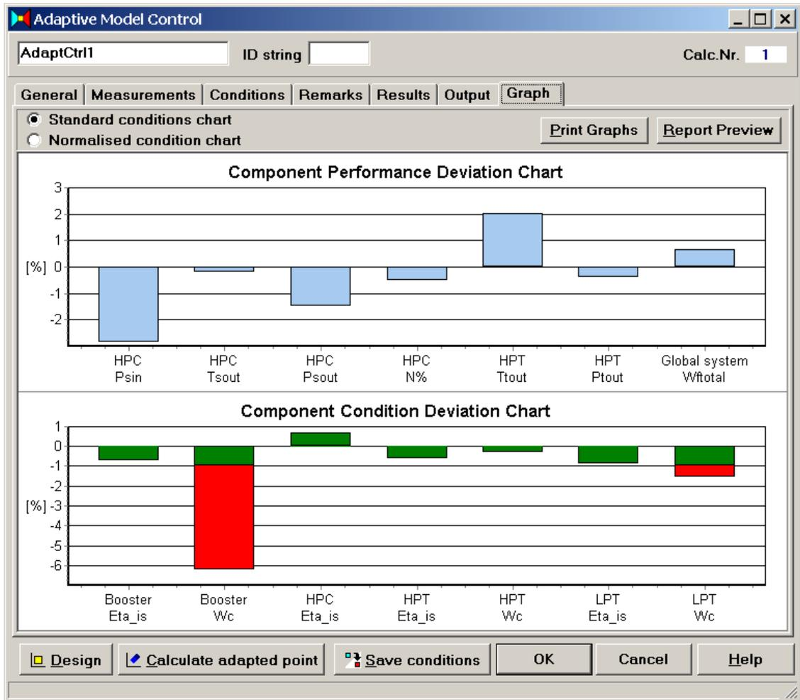
Figure 8 Gas path analysis results chart window, case 1
