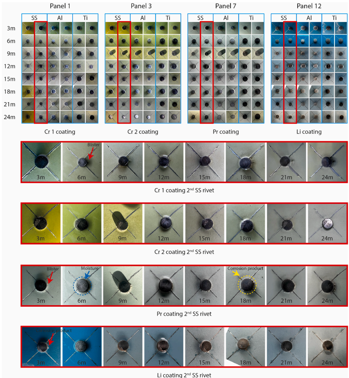
Fig. 6. Visual inspection results of outdoor exposure test panels with detailed images showing corrosion progression over time around X-scribed stainless-steel rivets for chromium, praseodymium and lithium coating systems.
