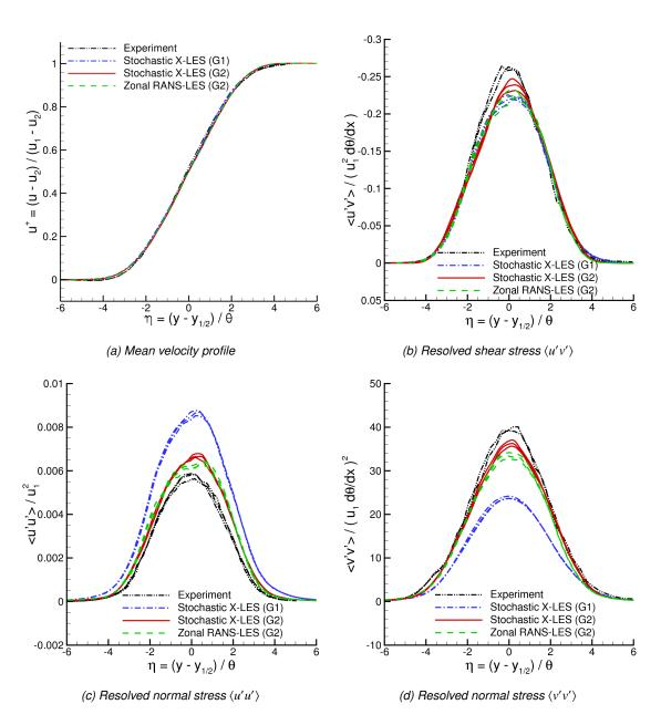
Fig. 3 Self-similar solution for X-LES and zonal RANS–LES computations of plane shear layer compared to experiment of Delville (Ref. 2).
