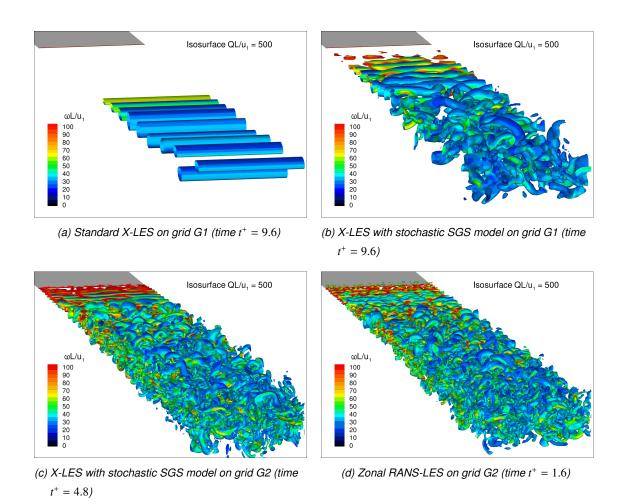
Fig. 2 Instantaneous isosurfaces of  $Q = \omega^2 - S^2$ , coloured with vorticity magnitude  $\omega$ , for X-LES and zonal RANS–LES computations of plane shear layer (S is magnitude of rate-of-strain).
