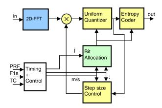
Fig. 3 FFT-ECBAQ Block diagram
