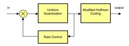
Fig. 2 ECBAQ block diagram
