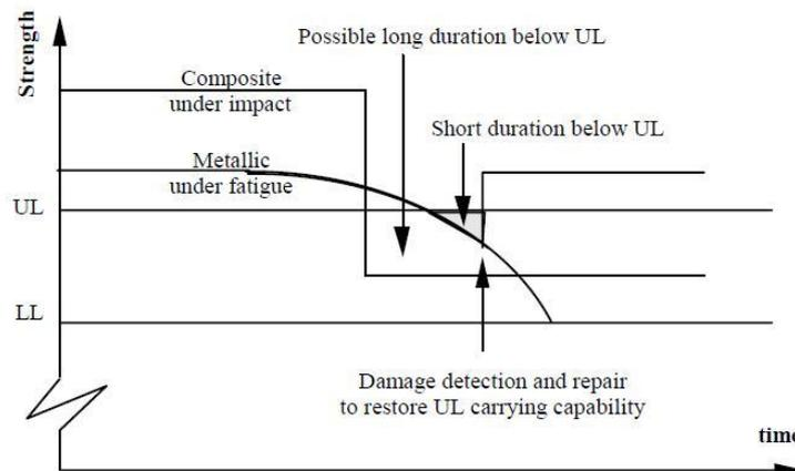
**Fig. 2 Comparison of composite non-growing damage and metal fatigue crack damage (Ultimate Load, UL, and Limit Load, LL) (Fig. 7.2.2.2c from [1])**
