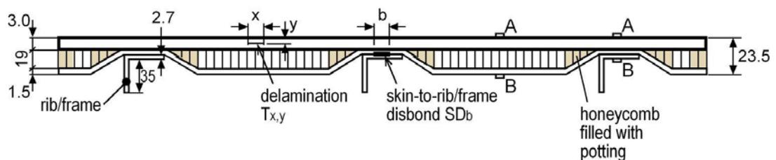
Fig. 3 Chamfered sandwich structure with 3 L-shaped ribs/frames
