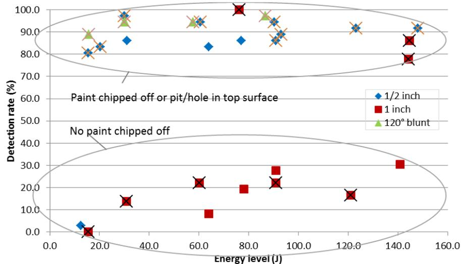
**Fig. 10 Overview of the detection rate for different impactors used on 20 mm thick, painted RTM specimens. An X through a point denotes a high speed impact (Fig. 16 from [6])**
