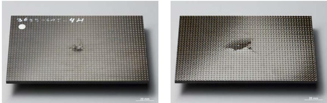
**Fig. 6 Impact on a thin laminate. Left: dent caused by a 16 mm spherical impactor at 21 J. Right: outbreak at the back of the same sample (Fig. 2 from Ref. 6)**
