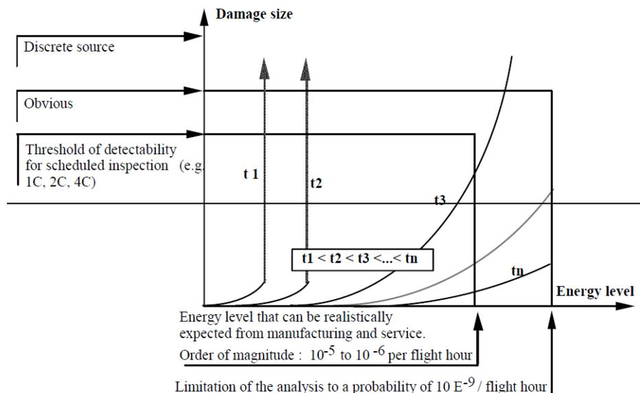
**Fig. 7 Damage size versus impact energy level for composite structures of different thickness  $t$  (Fig. 7.2.2.2(b) from [1])**
