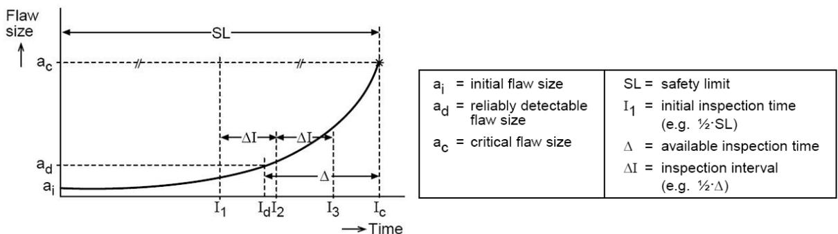
**Fig. 1 Damage tolerance approach for inspectable structures (Fig. 1 from [2])**
