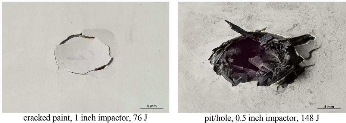
**Fig. 8 Readily detectable high-velocity impact damages on 20 mm thick, painted RTM specimens [6]**
