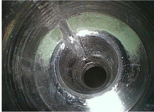
Figure 47: Non-perpendicular saw cut.
