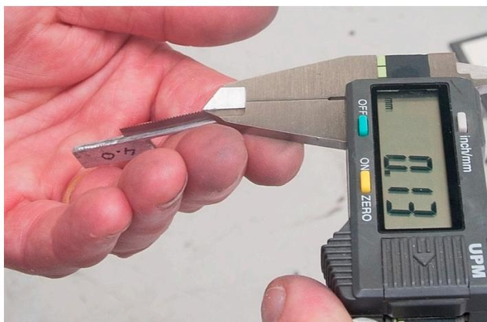
Figure 46: Sawblade thickness.
