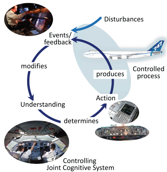
Fig. 1. The cyclical model of human action and perception, conceptually applied to the crew-automation JCS (adapted from Hollnagel & Woods, 2005).
