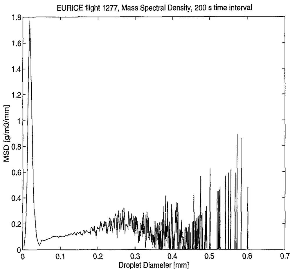
*Fig. 5 Droplet mass density distribution for droplets measured in the flight on 16 March 1997 in a 200-second time interval. The maximum mass density is for droplets of 19 micrometer, the MVD is 214 micrometer.*
