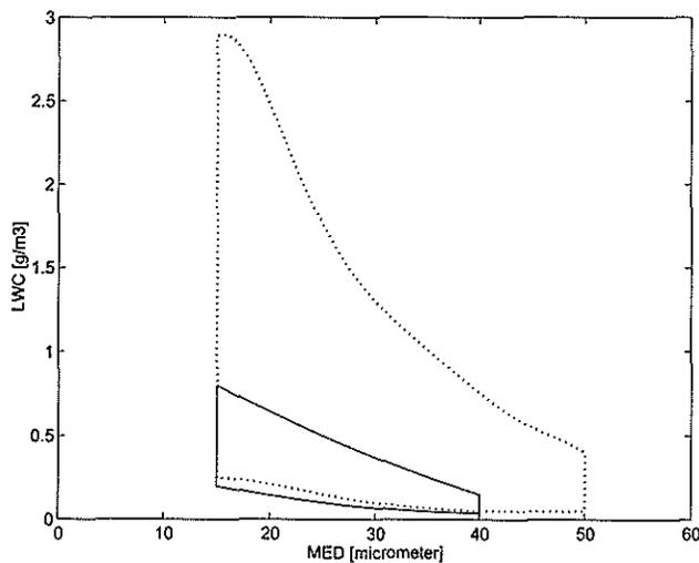
Fig. 4 Envelopes of MED and LWC ranges for the continuous cloud (-) and intermittent cloud (...) limits described in JARIFAR 25/29 Appendix C icing conditions. Within these envelopes additional limits are set for temperature and altitude. The complete description is given in ref. 2
