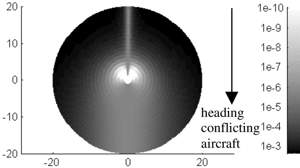
Figure 7: Overlap probability (with threshold reduced to 50 m) is represented by colours for various path angles and times to minimum predicted separation.
