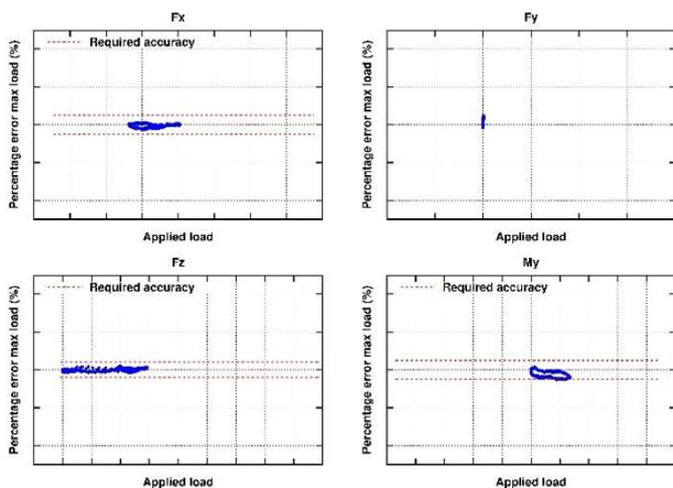
**Figure 17.** Relative percentage load error  $(F_{comp}-F_{exp})/maxload*100\%$  for the dynamic test at room temperature, red dashed lines is the required Airbus accuracy.
