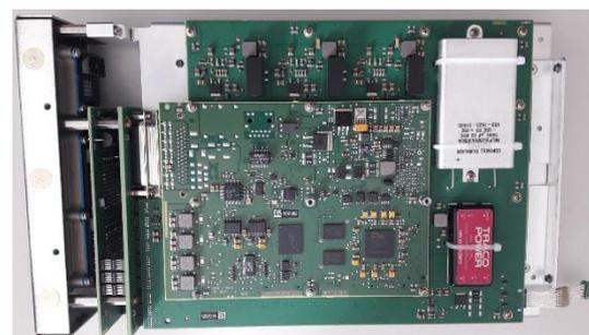
**Figure 6.** FOPU prototype - Digital processing part.
