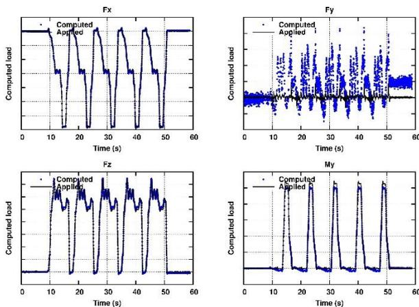
**Figure 16.** Comparison computed versus applied loads for the dynamic test at room temperature.
