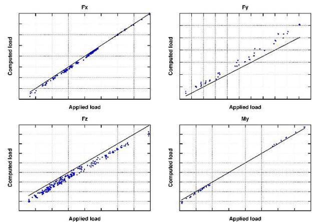
**Figure 24.** Comparison computed against applied loads at 20% LL at  $110 \text{ }^\circ\text{C}$ .
