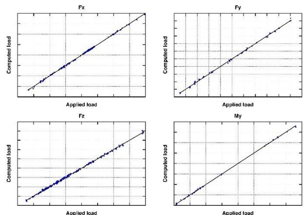
**Figure 15.** Comparison computed against applied loads at 20% LL RT.
