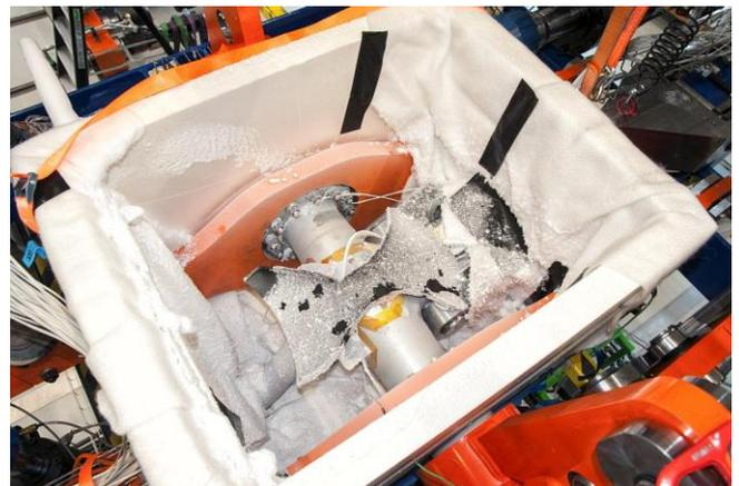
**Figure 12.** Climate chamber at the centre part of the MLG.
