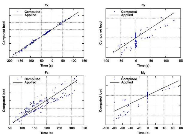
**Figure 20.** Comparison computed against applied loads at 90% LL at room temperature.
