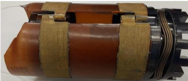
**Figure 7.** Axle sensor prototype, including clamping mechanism.
