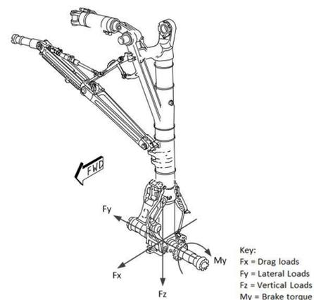
**Figure 1.** Landing gear load convention.
