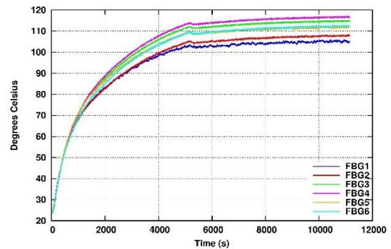
**Figure 22.** Temperature change at the FBG locations during heating of the axle.
