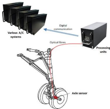
**Figure 3.** High-level overview of the optically-based landing gear load sensing and monitoring system.
