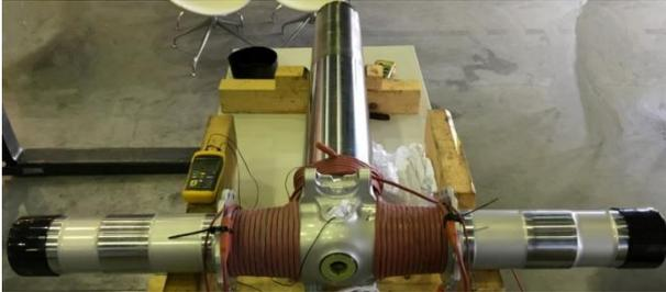
**Figure 9.** Main landing gear slider tube with installed heater bands.
