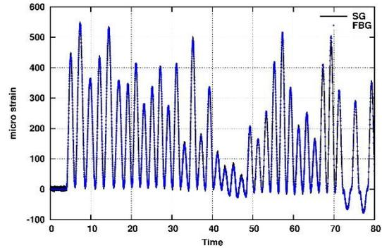
**Figure 14.** Strain gauge and FBG response comparison for 20% LL.
