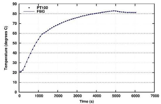
**Figure 21.** FBG8 and PT100 temperature response during warmup to 80 °C.
