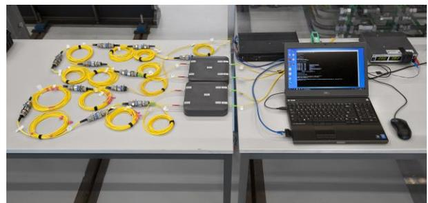
**Figure 8.** FOPU and part of the optical cables (without final harnessing) and connectors.
