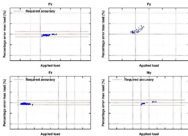
**Figure 25.** Relative percentage load error ( $F_{comp}-F_{exp}$ )/ $\max load * 100\%$  at 20% LL 110 °C, red dashed lines is the required Airbus accuracy.
