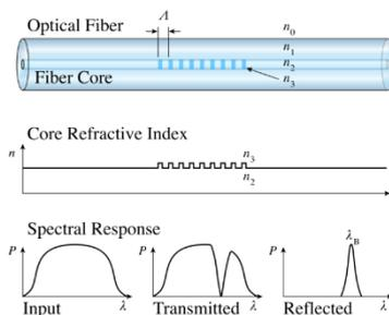
**Figure 2.** Principle of a Fibre Bragg Grating sensor, from Wikipedia.
