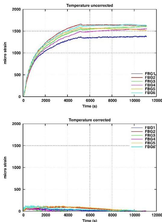
**Figure 23.** Temperature uncorrected (top) and corrected (bottom) FBG strain responses during warmup to  $120 \text{ }^\circ\text{C}$ .
