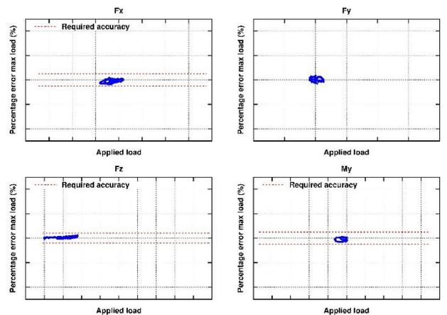
**Figure 19.** Relative percentage load error  $(F_{comp}-F_{exp})/maxload*100\%$  for the flight profile at room temperature, red dashed lines is the required Airbus accuracy.
