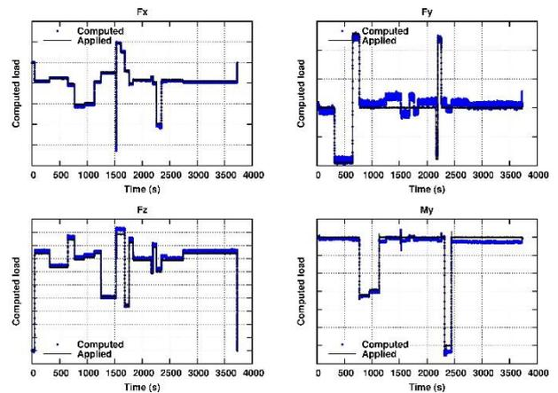
**Figure 18.** Comparison computed versus applied loads for the flight test at room temperature.
