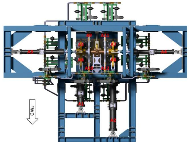
**Figure 11.** Top view test rig with indicated actuator locations.
