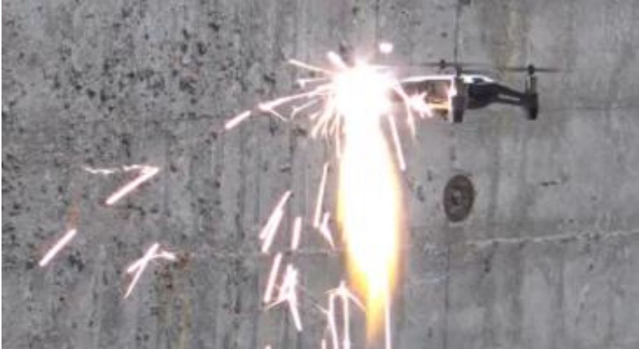
Figure 5: Laser engagement of a DJI Tello drone.
