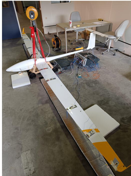
Figure 6. Ground vibration testing setup.
