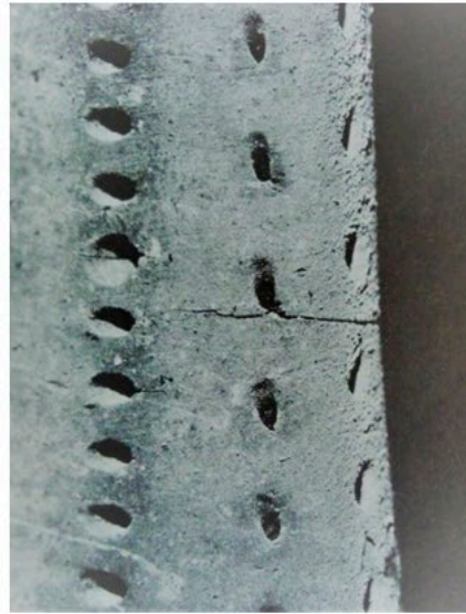
Detail of crack formation in leading edge of 1 st stage turbine blade
