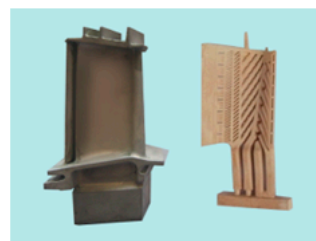
Example of casted blade and ceramic insert
