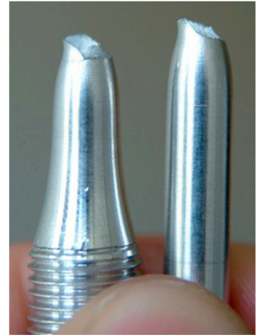
Round bar tensile specimen after testing
