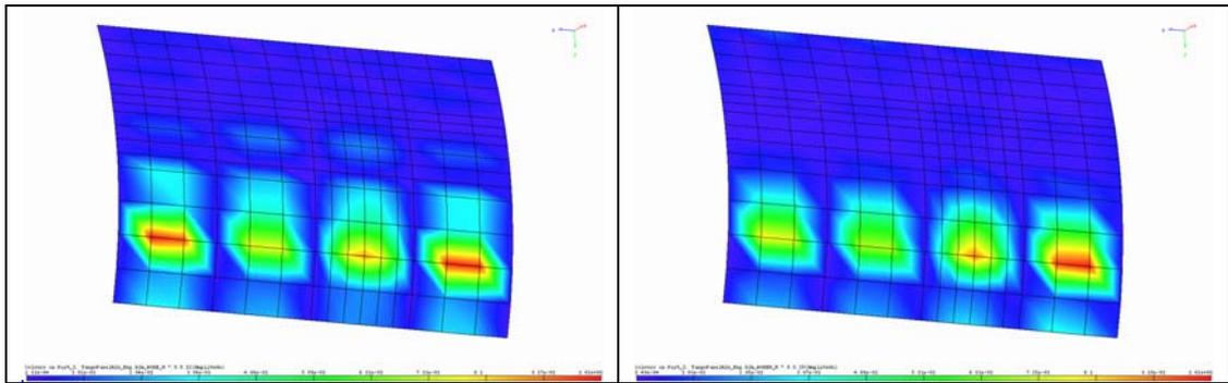
Figure 3.8: Experimental (left) versus numerical (right) mode shape on the experimental grid: mode 12
