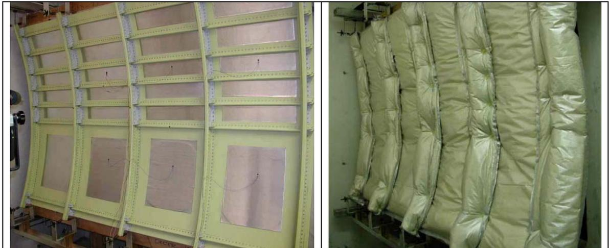
Figure 3.1: Damped (left) and furnished (right) Aluminium fuselage panel
