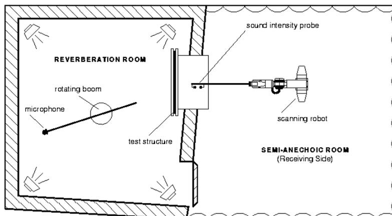
Figure 3.2: Schematised measurement set-up, from Ref. 7
