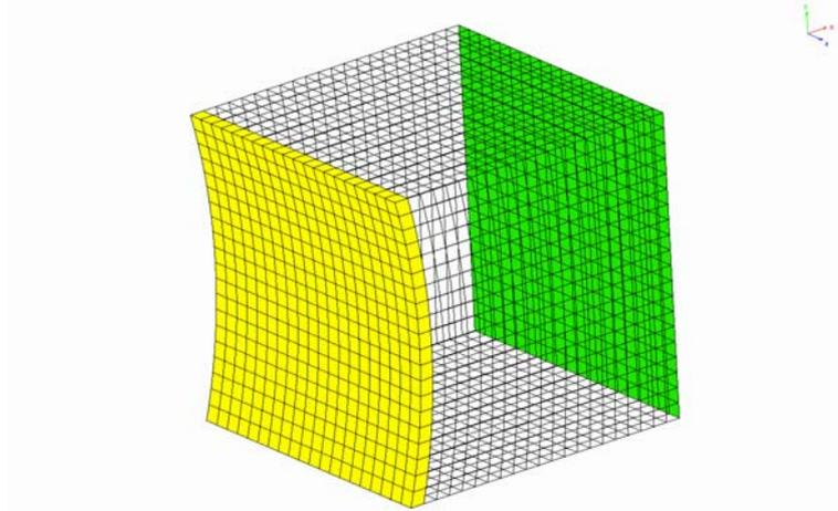
Figure 3.10: FEM model Duct with glass wool layer (yellow) and impedance boundary condition (green)
