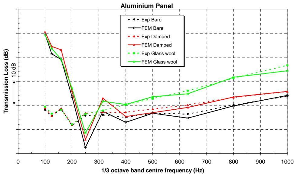
Figure 3.13: Experimental (dotted) and numerical (solid) TL-curves for Aluminium panel configurations: bare, damped and furnished
