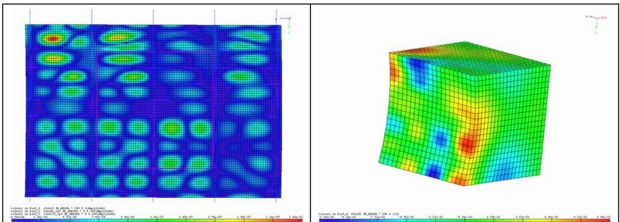
Figure 3.11: Response at 414 Hz for: panel displacement (left) and resulting fluid response in duct (lower right)
