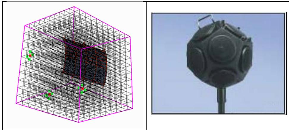
Figure 3.3: Left: FEM model of reverberant room including the FEM model for the Aluminium fuselage panel. Red spots are the dodecahedron source positions. Right: dodecahedron.
