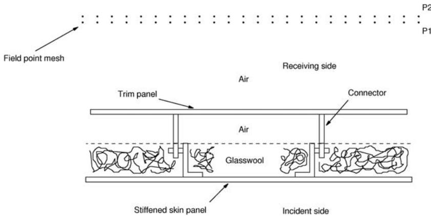
Figure 1.1: Schematised double wall set-up
