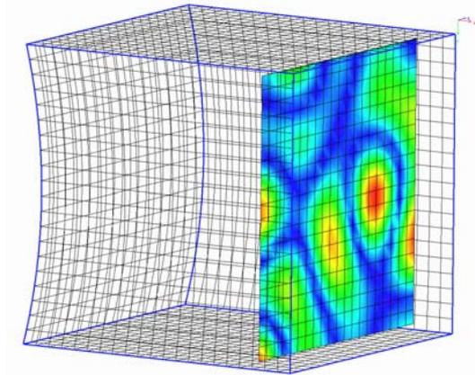
Figure 3.12: Calculated sound field at 836 Hz on the field point mesh: real part of the total pressure
