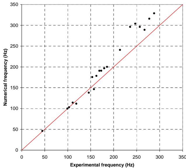
Figure 3.9: Numerical versus experimental eigenfrequencies for Aluminium panel
