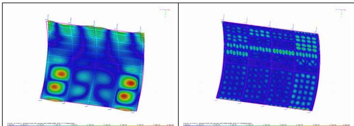
Figure 3.7: One of the lowest (17<sup>th</sup>) and highest mode shapes (390<sup>th</sup>).
