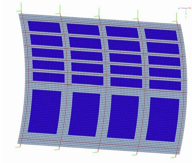
Figure 3.6: FEM mesh of the damped Aluminium panel: shells (light blue), beams (red) and rods (green). The dark blue elements represent the constrained layer damping.
