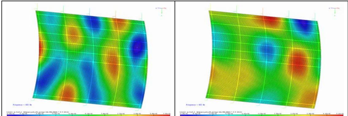
Figure 3.4: Complex frequency dependent pressure distribution at the panel, real (left) and imaginary (right) part, for 402 Hz
