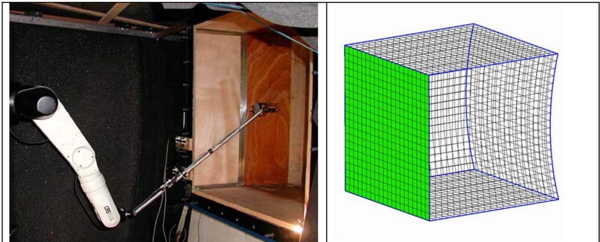
Figure 3.5: Sound intensity measurement set-up (left) and FEM mesh of duct with impedance boundary condition (green) representing the end-plane
