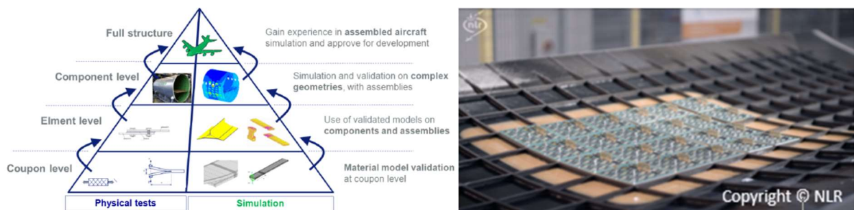
Figure 1: Pyramid of testing (left) [17], a picture of the full-scale panel including the antenna's (right).
