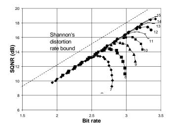
Fig. 1 SNQR of ECSQ as a function of the output entropy for a Gaussian IID source  $\sigma$  with =0.25
