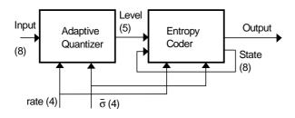
Fig. 3 Architecture of a fast ECBAQ encoder
