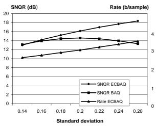
Fig. 2 SNRQ of ECBAQ and BAQ both optimised for  $\sigma$  = 0.2, 3 b/s, as function of the signal's standard deviation
