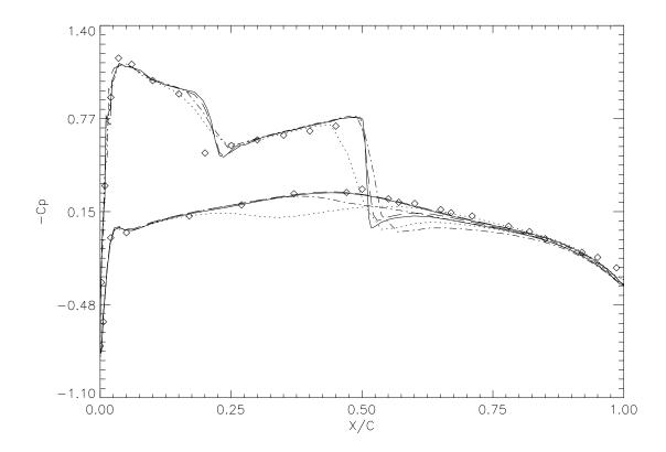
Figure 11: Pressure coefficient  $C_p$  at cross-section y = 0.65S of ONERA M6 wing,  $M_{\infty} = 0.84, \alpha = 3.06^{\circ}$  (··· original grid, — - — one adaptation, — — two adaptations, — — three adaptations,  $\diamond \diamond \diamond$  experiment).
