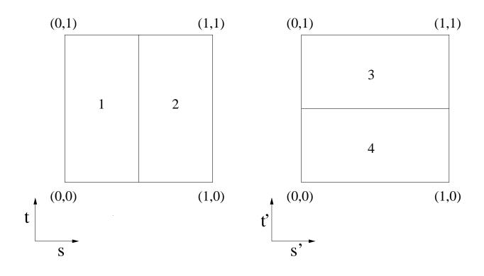
Figure 2: Element refinement at left and right side of elementary face. Elements 1 and 2 can not be connected to elements 3 and 4 with one face.
