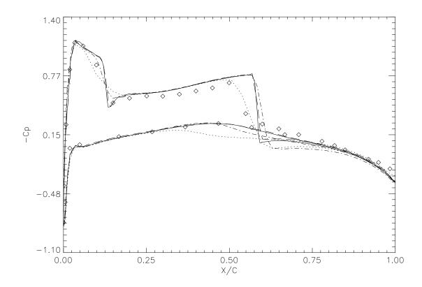
Figure 10: Pressure coefficient  $C_p$  at cross-section y = 0.44S of ONERA M6 wing,  $M_{\infty} = 0.84, \alpha = 3.06^{\circ}$  (··· original grid, — - — one adaptation, — — two adaptations, — — three adaptations,  $\diamond \diamond$  experiment).
