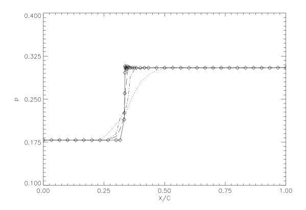
Figure 5: Pressure distribution along a 10° ramp for supersonic flow,  $M_{\infty} = 2.0$  (··· original grid, — - — two adaptations, — — four adaptations, —— six adaptations,  $\diamond \diamond \diamond$  final adapted grid).
