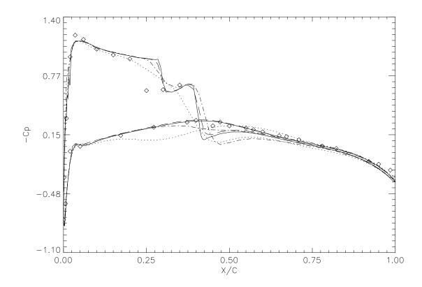
Figure 12: Pressure coefficient  $C_p$  at cross-section y = 0.80S of ONERA M6 wing,  $M_{\infty} = 0.84, \alpha = 3.06^{\circ}$  (··· original grid, — - — one adaptation, — — two adaptations, — — three adaptations,  $\diamond \diamond \exp($  experiment).
