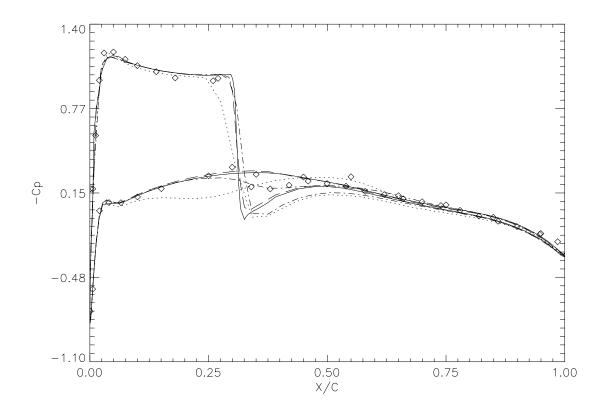
Figure 13: Pressure coefficient  $C_p$  at cross-section y = 0.90S of ONERA M6 wing,  $M_{\infty} = 0.84, \alpha = 3.06^{\circ}$  (··· original grid, — - — one adaptation, — — two adaptations, — — three adaptations,  $\diamond \diamond \exp($  experiment).
