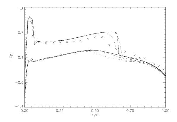
Figure 9: Pressure coefficient  $C_p$  at cross-section y = 0.20S of ONERA M6 wing,  $M_{\infty} = 0.84, \alpha = 3.06^{\circ}$  (··· original grid, — - — one adaptation, — — two adaptations, — — three adaptations,  $\diamond \diamond \diamond$  experiment).
