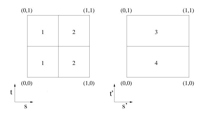
Figure 3: Faces of elements 1 and 2 are split into sub-faces such that each sub-face connects to one element at each side.
