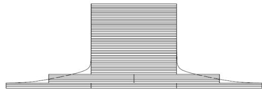
Figure 5: Trapezoid rib shape with layer build up
