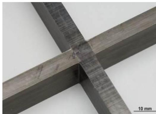
Figure 2: Rib stiffening crossing section sample manufactured at NLR [4]
