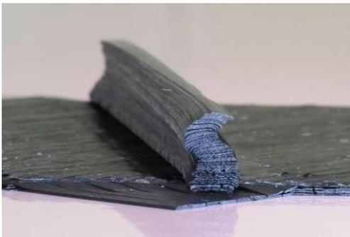
Figure 12: First rib height trial showing unstable behavior above 15 mm rib height.
