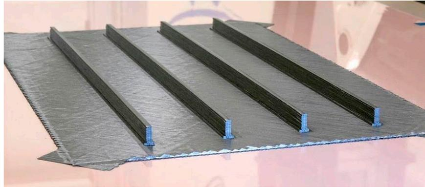
Figure 21: Fibre placed panel with skin and four ribs before autoclave cure
