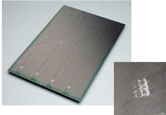
Figure 31: Cured SLM mesh panel.
