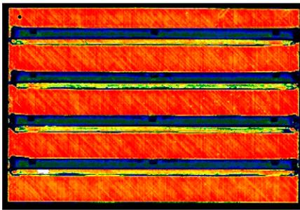
Figure 32: Attenuation C-scan of SLM panel skin
