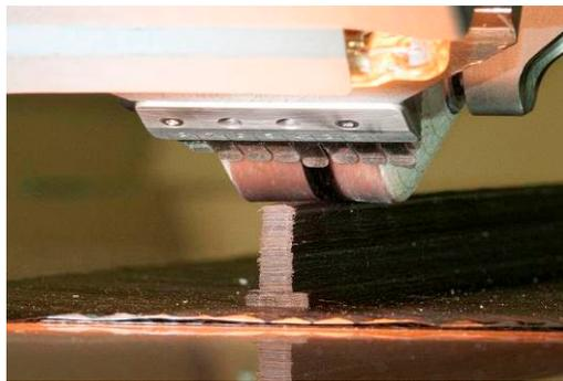
Figure 11: Rib manufacturing using fibre placement without support during fibre placing
