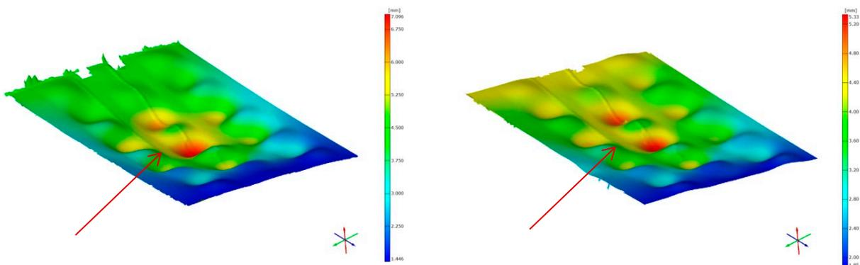
Figure 35: Displacement of panels during compression test measured using digital image correlation of RHEA mesh panel (left) and SLM mesh panel. View of outer skin side. The red arrow points at the mesh position.
