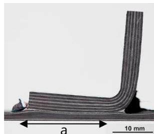
Figure 34: Rotated L-stiffener of panel with SLM meshes.
