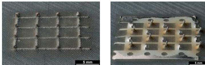
Figure 16: Detail of embedding using 50 Shore rubber sheet
