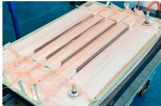
Figure 29: Finished vacuum bag with grips
