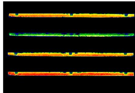
Figure 33: Attenuation C-scan of SLM panel stiffener-skin bond
