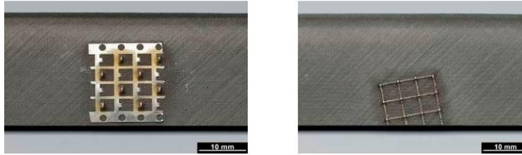
Figure 26: Embedded meshes in stiffeners.
