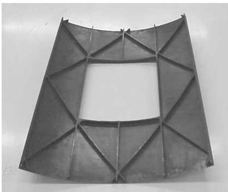
Figure 1: Grid stiffened panel from the Minotaur payload fairing [6]
