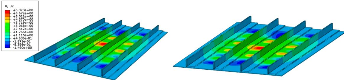
Figure 18: Rib stiffened panel buckling mode (left) and blade stiffened panel with out of plane buckling displacements (right)
