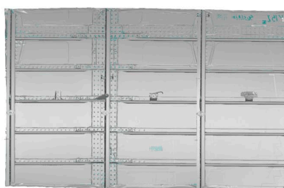
Figure 23: Surface mesh of the back side of both panels obtained by 3D scanning (mirrored such that it corresponds to the optical photographs)
