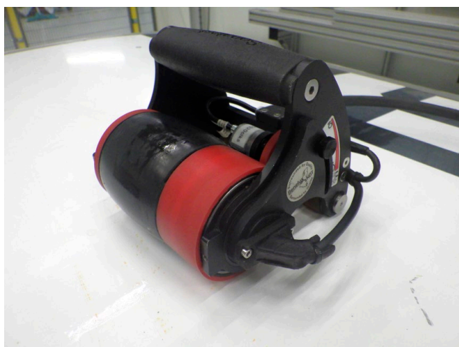
Figure 10: Sonatest Wheel probe with 5L64 PAUT transducer
