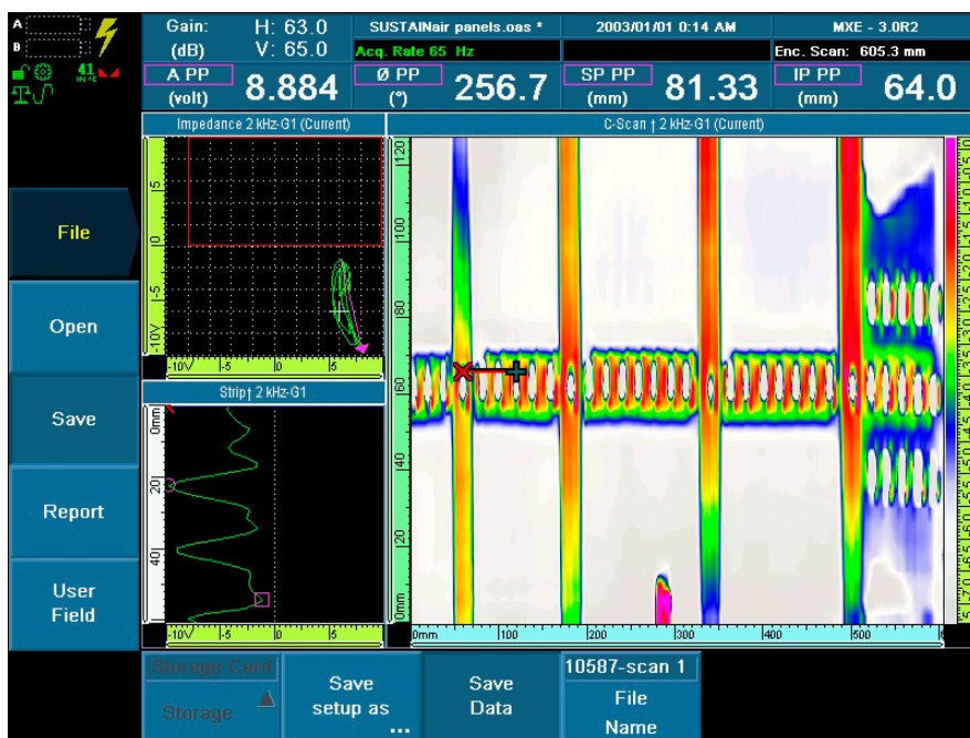
Figure 27: ECA result of stringers and rivet row of panel 10587 (not scaled in the scan axis)
