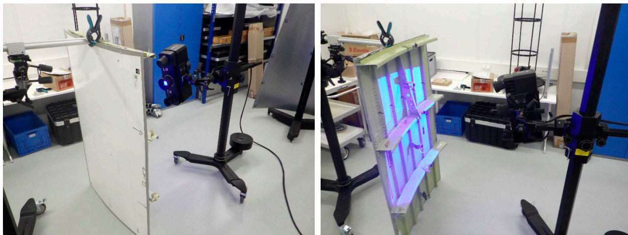
Figure 21: Photographs of the 3D scanning of panel 10597
