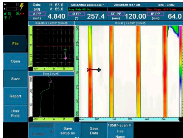
Figure 5: Example of a typical C-scan image of stringers under the skin of the panel (not to scale)
