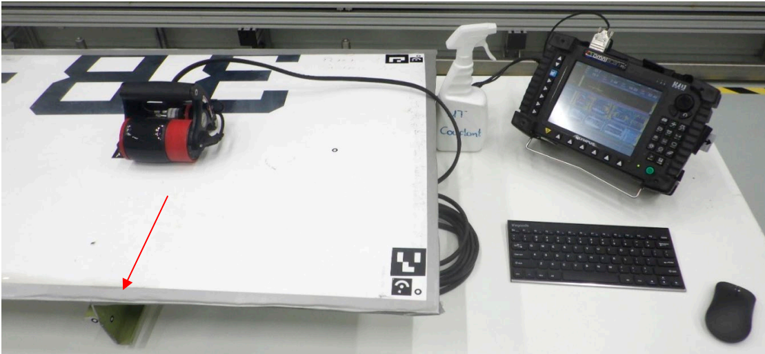
Figure 29: PAUT inspection on panel 10587 with the red arrow indicating the scan direction
