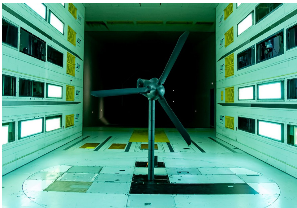
Fig. 1 ATTILA testbed in the DNW Large Low-speed Facility (LLF) 6 m × 6 m wind tunnel test section
